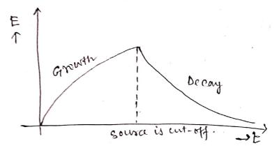
Let The time taken to reduce the energy density and therefore intensity to de cary by 60 db i.e. I millionth part of the value just before cut-off. Therefore.
